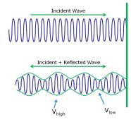
between the high and low voltage in the transmission line is the Voltage Standing Wave Ratio. The log version of VSWR is called Return Loss.
