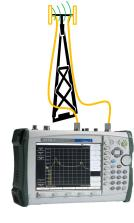
The **setup** for antenna isolation tests uses the BTS Master, Cell Master, or Site Master's Two Port Insertion Loss capability. After a two port calibration (An OSLIT cal), the signal source is connected to one antenna while the sense terminal is connected to the
