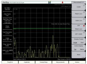
DTF is a way to locate faults identified by Return Loss or VSWR measurements.
