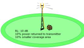
Reduced coverage increases dropped and blocked calls due to weak signal areas and network loading imbalances.
