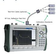
**OSL** is the most accurate calibration for one port tests such as Return Loss, VSWR, and DTF. An OSL calibration requires the use of three precision standards, and is as accurate as the standards.
