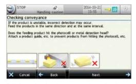
Built-in troubleshooting screens determine the cause of false rejects and provide suggestions to ensure repeatable, stable system performance.
