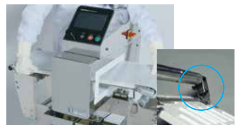
Tool free belt removal
