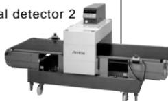
\*1 The metal detector is best positioned at the last stage before delivery of the product to the consumer.
