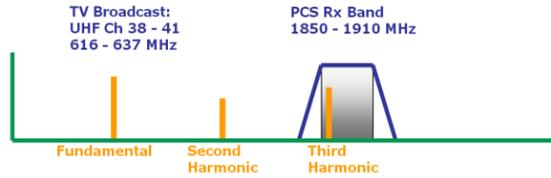
Sometimes harmonics become much worse than the legal limit. For instance, a transmitter with a class B output stage may lose a transistor, only amplifying half of the signal. This will produce a “Picket Fence” array of harmonics across the spectrum.
