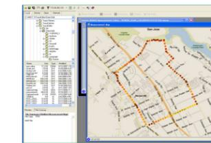
the Master series instruments have a GPS option, it's possible to hunt down interference by recording an interference signal's power
