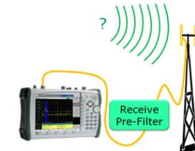
**Frequency Division Duplex (FDD)** base stations, such as GSM, CDMA, and W-CDMA, can use the spectrum analyzer’s channel power measurement, but use it at the receive frequency. This approximates the switch’s Rx noise floor measurement. The measurement must be made during a quiet time when no calls are up. The same screen also normally has occupied bandwidth, to aid in signal identification.
