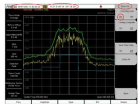
simplify stand-alone signal monitoring. It is very useful when a LAN is not available. The best way to create a Save-on-Event mask is to first collect a max-hold waveform
