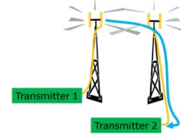
**Shared antennas** can create IM if the antenna or antenna cable run is corroded.
