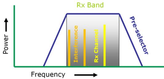
The unwanted, or interfering, signal does not need to be on the receive channel. If strong enough, it only needs to be within the radios’ Rx duplexer or pre-selector frequencies.
