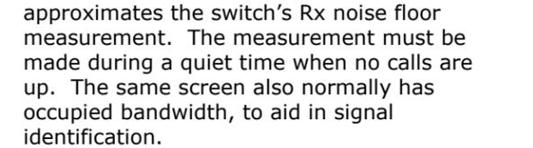
**Time Division Duplex (TDD)** systems, such as TD-SCDMA and WiMAX can use the gated power measurement on the Power vs. Time screen to approximate the switch Rx noise floor measurement. Again, the Rx noise floor measurement must be made during a quiet time, when no calls are up.
