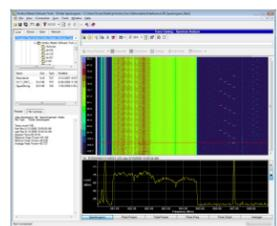
Like the spectrum analyzer based spectrogram, it is a great help when looking for weak signals, drifting carriers, or hopping signals. When loaded with the
