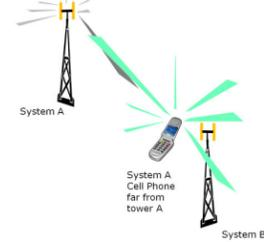
If a cell phone is a long ways from its tower, it will be transmitting at high power. If, at the same time, it is near another operator’s tower, one it cannot hand off to, it may be transmitting within the other base station’s pre-selector and cause de-sense. Near Far problems can be reduced by co-location.
