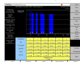
**Channel Scanners** work on any signal and are useful when looking for IM or harmonics. They can help spot signals widely separated in frequency that turn
