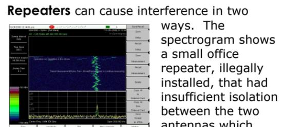
A different repeater issue comes up when a network operator installs a large area repeater that unintentionally amplifies other operator’s signals. This can lead to unexpected excess coverage problems and frequency re-use issues.
