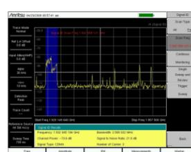
decoded call sign. The Master series of spectrum analyzers has a Signal ID option which takes much of the mystery out of the spectrum.
