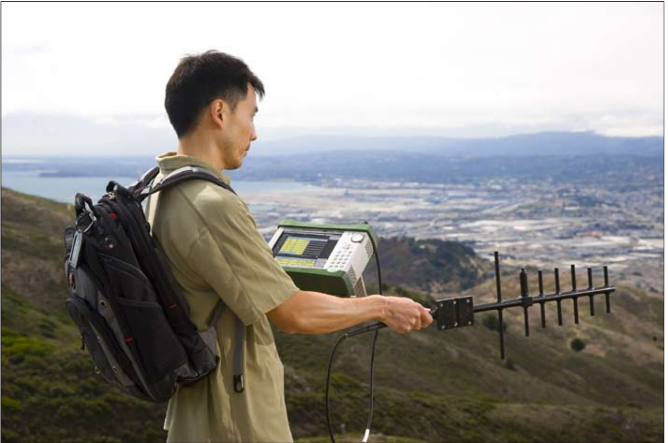
Figure 5. Performing EVM measurements with Yagi antenna.
